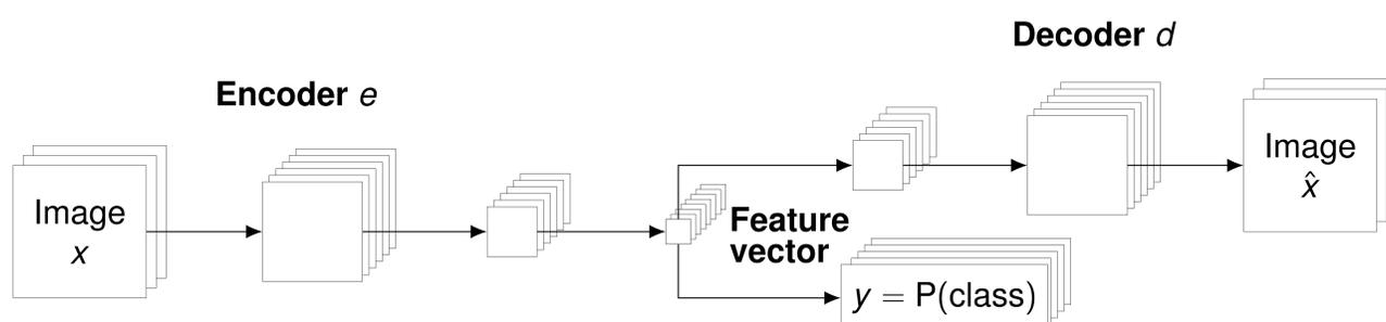
The encoder is trained for the supervised task. The decoder is trained as an identity function.
